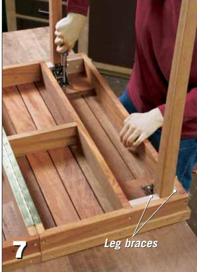
**7** *Fasten the legs and leg brackets with the tapered sides facing toward the inside. Then fasten the brackets to the leg cleats. The legs should fit snugly between the leg braces.*
