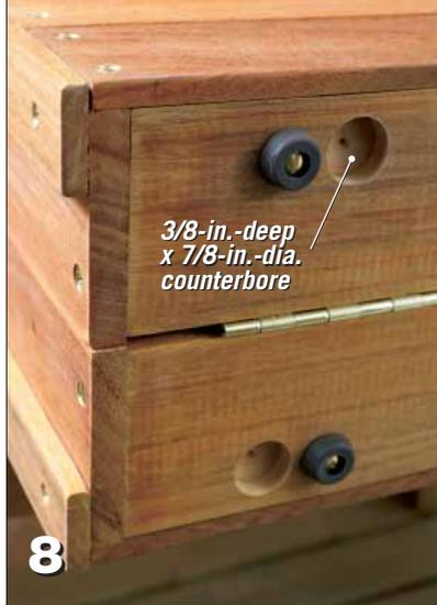
**8** *Offset the four rubber feet and counterbores so that when the table is opened each foot will fit into a counterbored recess. Use a 7/8-in.-dia. Forstner bit to bore the recesses.*
