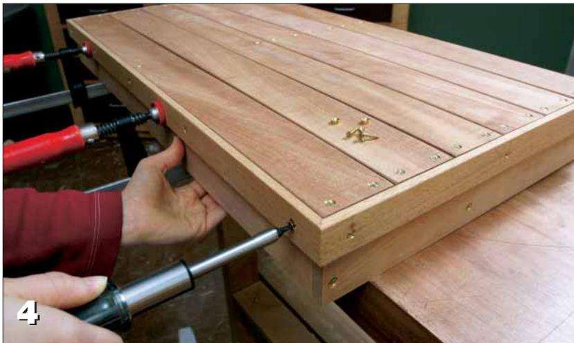
**4** Attach the top slats and trim rails with No. 6 x 1-in. brass screws and countersunk washers. A ratcheting screwdriver works well for driving the slotted screws.
