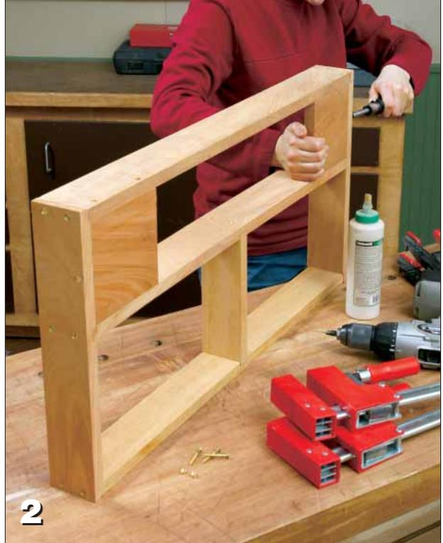
**2** Glue and clamp the rails together. Drill a 1/8-in.-dia. pilot hole in the center of each counterbore, and fasten each joint with a No. 8 x 1-1/2-in. brass screw and countersunk washer.
