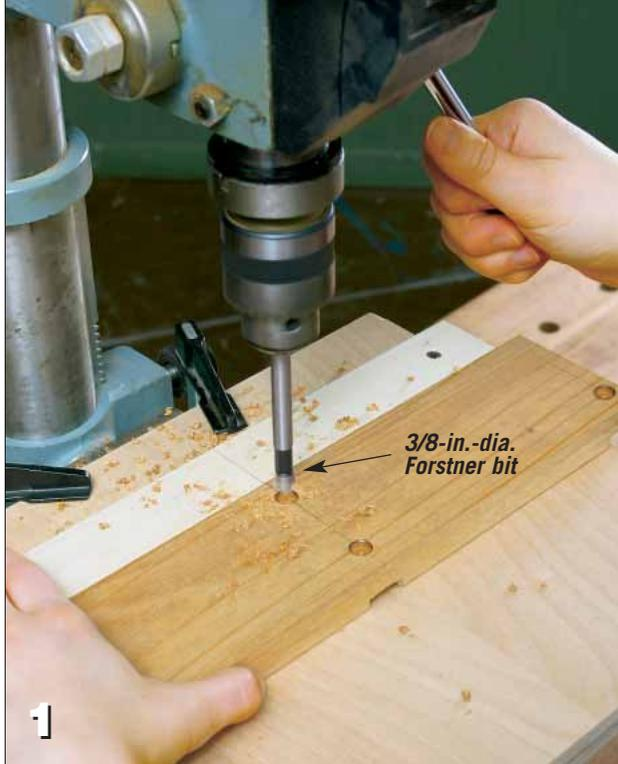
**1** Bore 3/8-in.-dia. x 3/16-in.-deep counterbores for the No. 8 countersunk washers. Mark the position of the Forstner bit's center on a fence to position the rails.
